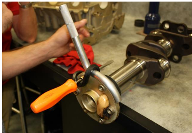
The Lycoming one-piece crank seal and the special tool that stretches it over the prop flange. The curved part of the lever is grooved to slide around the flange. Courtesy www.glasair-owners.com
