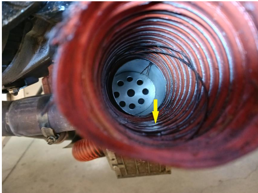
The cabin heat muff intake tube sits beneath the front crank seal. Arrow shows oil in the tube, which then gets into the heat muff and stinks up the cabin.
