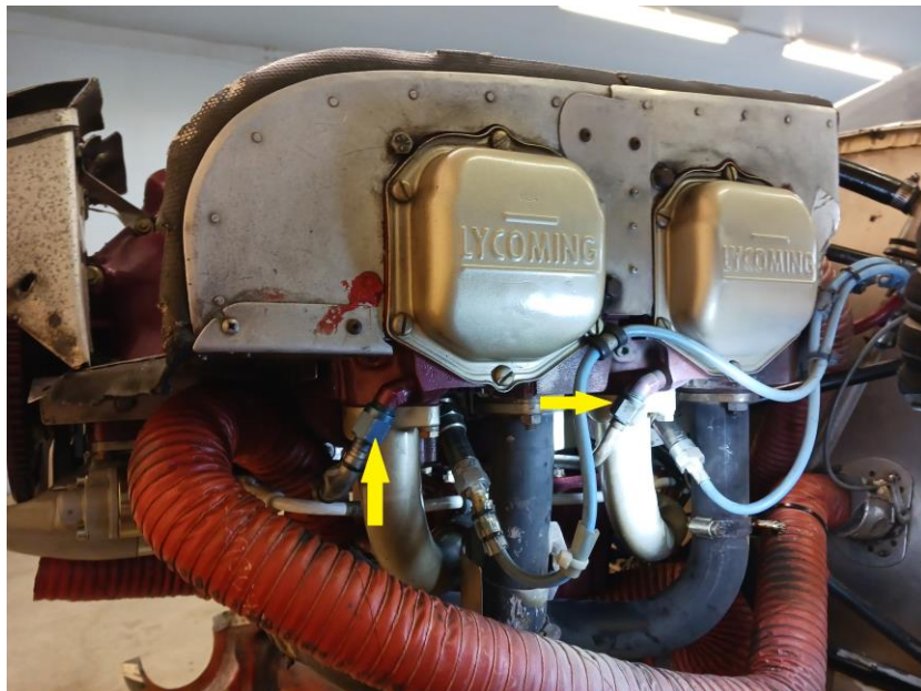
Arrows point to the cylinder head oil drain lines on cylinders #2 and #4.
