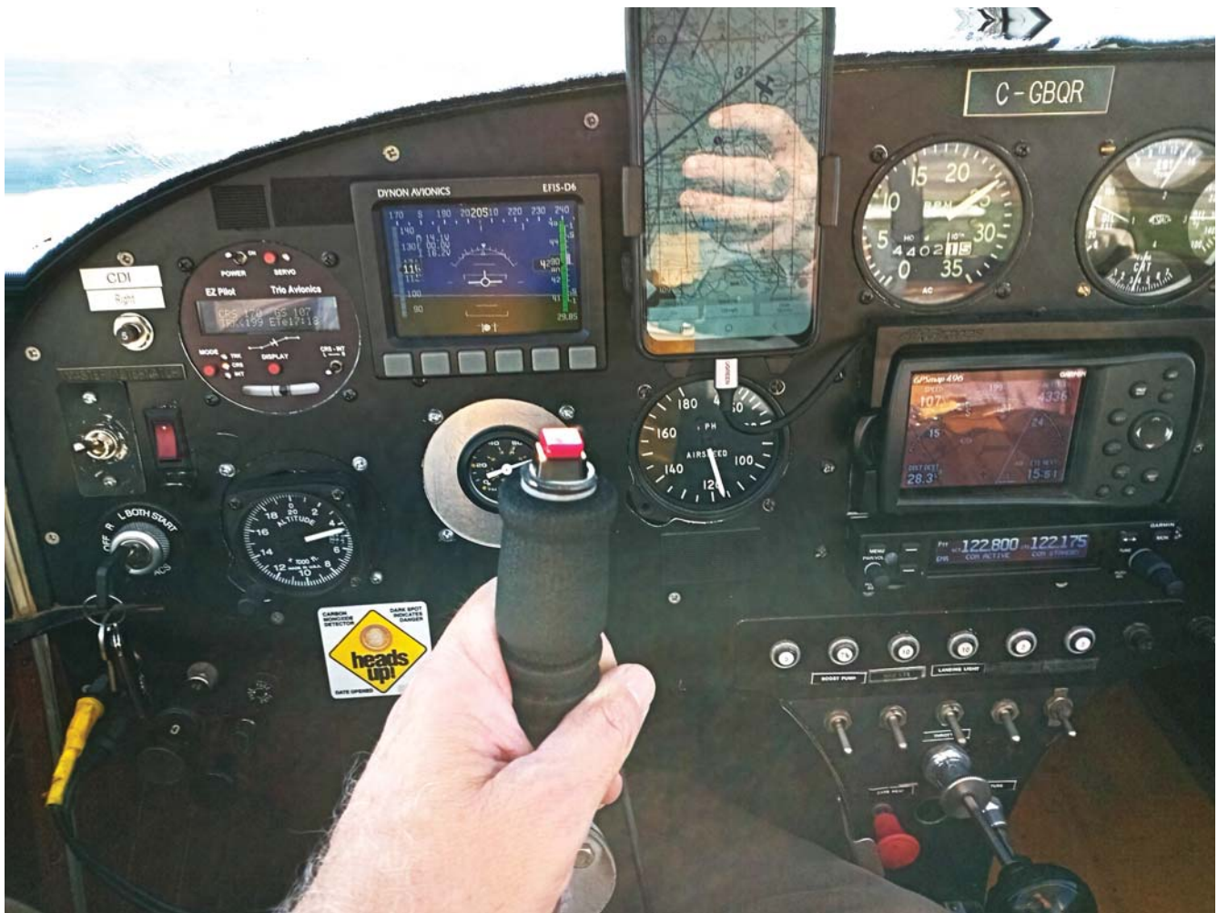
The Cav's panel. The EZ Pilot control head is left of the Dynon EFIS. A Garmin 496 is below the tachometer. By Stu Simpson.
