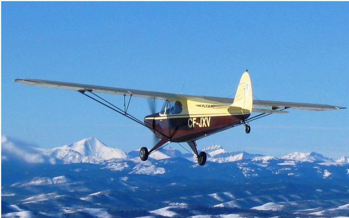
Kirkby's other Piper, the PA-12 Super Cruiser, which cruises at about 105 mph.
