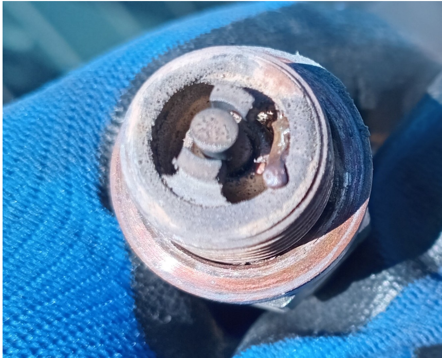
One of the front two lower spark plugs heavily fouled with lead deposits.
