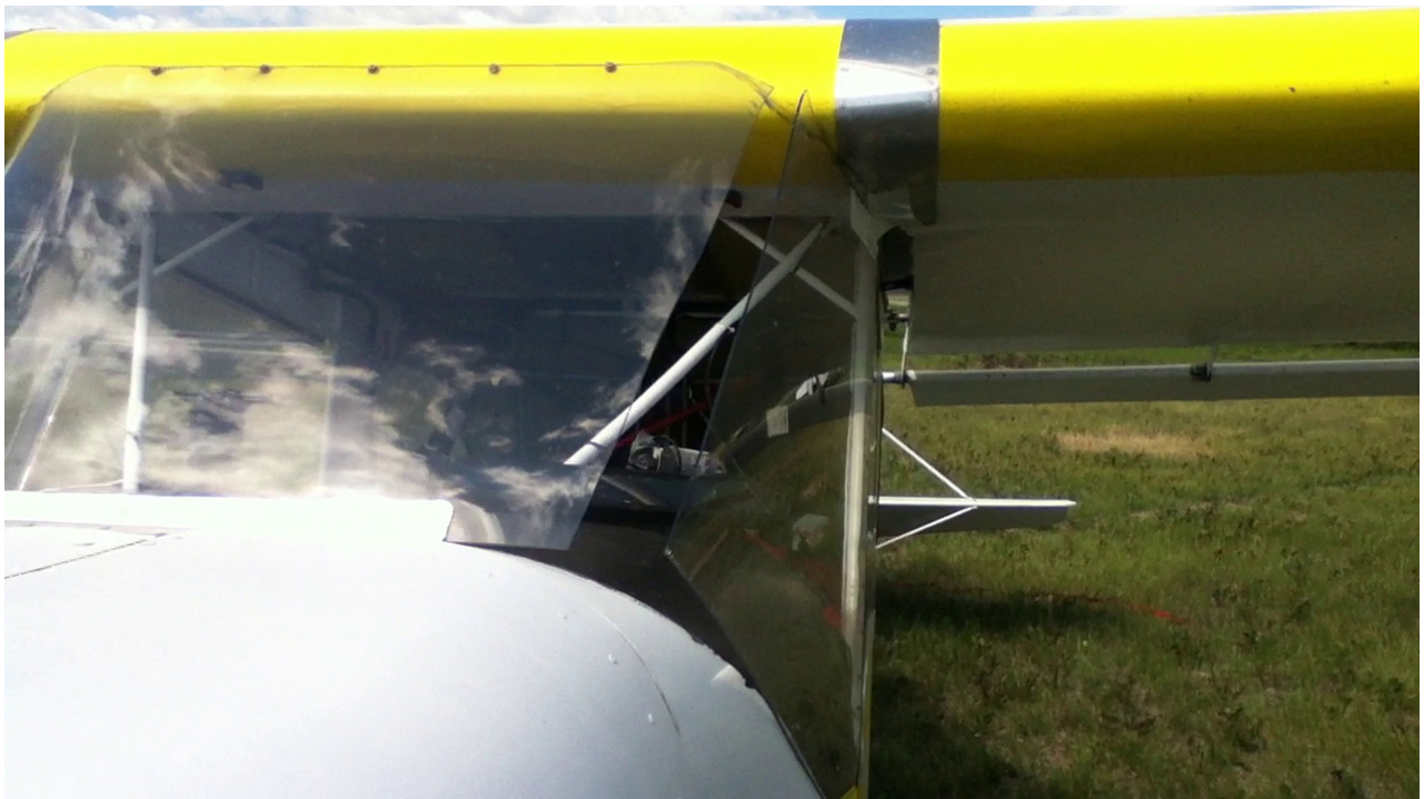
The Merlin's windshield snapped into two pieces.
