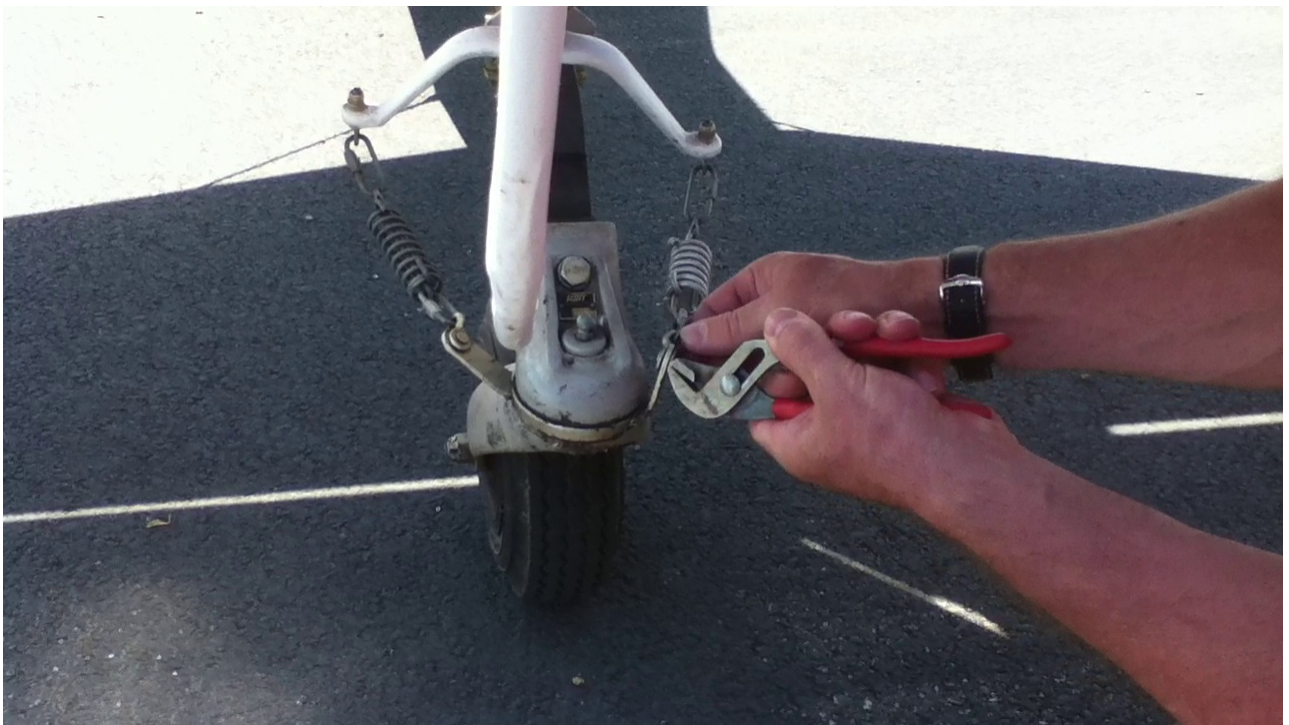
The bent steering control arm on the Champ; a very serious problem.
