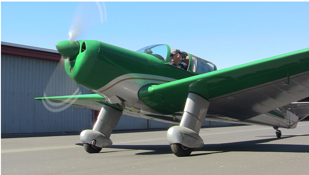
A Ryan SC-W, with a Continental E-185 engine instead of a radial.
