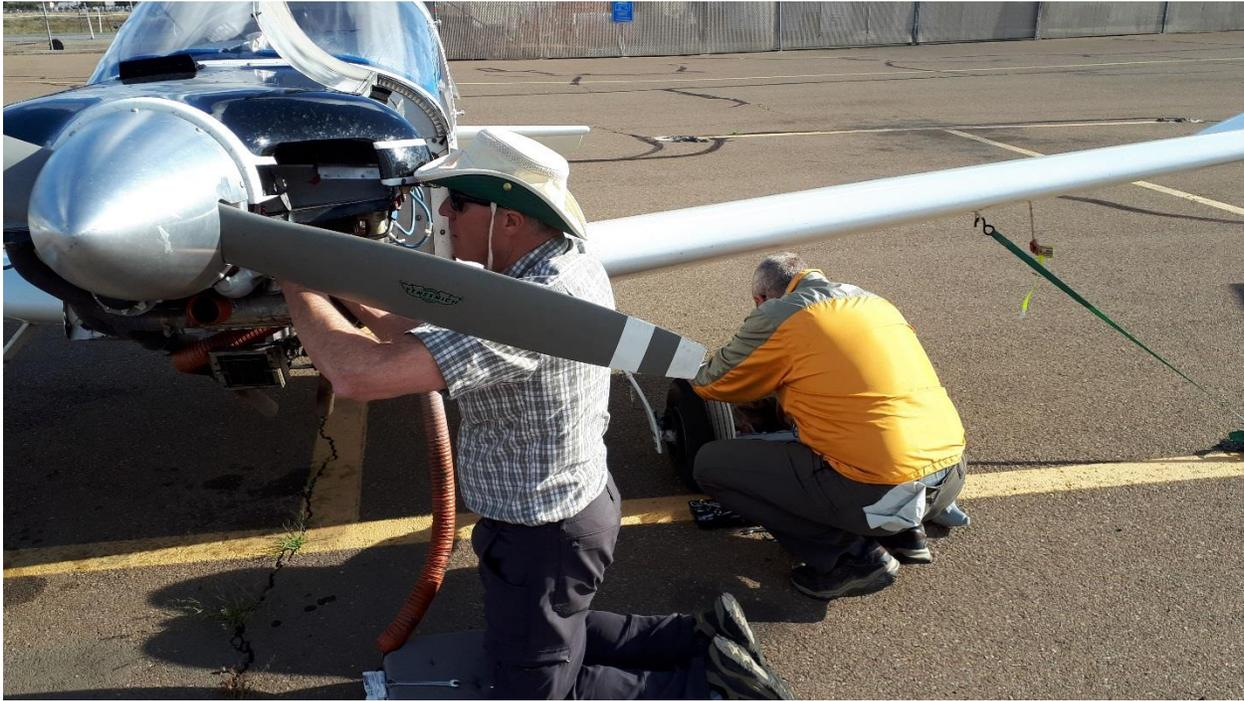
Replacing the Cav's starter solenoid at Gillespie Field. By Stu Simpson
