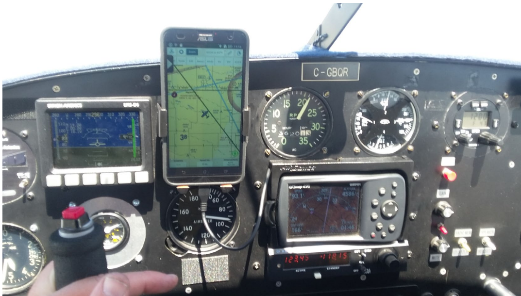
Cav Nav - The author's panel featuring a cell phone with Fltplan.go and a Garmin 496 dock-mounted GPS. By Stu Simpson
