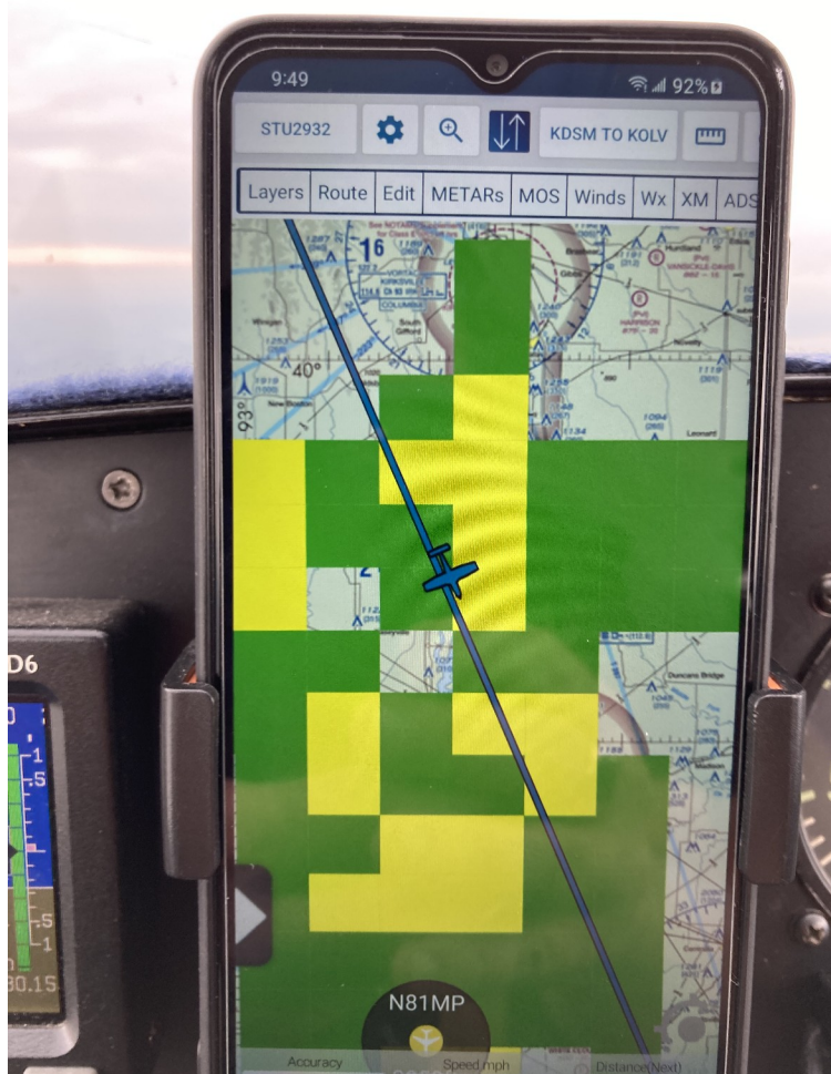
A radar image from ADS-B showing light precipitation along our route over Missouri. The round symbol toward the bottom of the photo is another aircraft. By Stu Simpson
