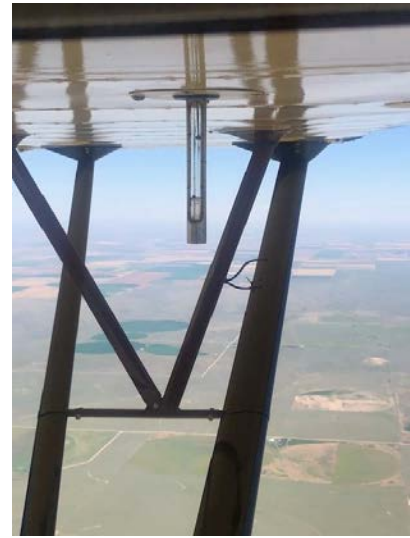
Figure 10. Water in the Sight Glass
