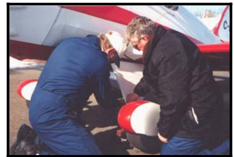
Bob and Glen re-assemble the Renegade wheel after changing tube. Photo by Stu.
