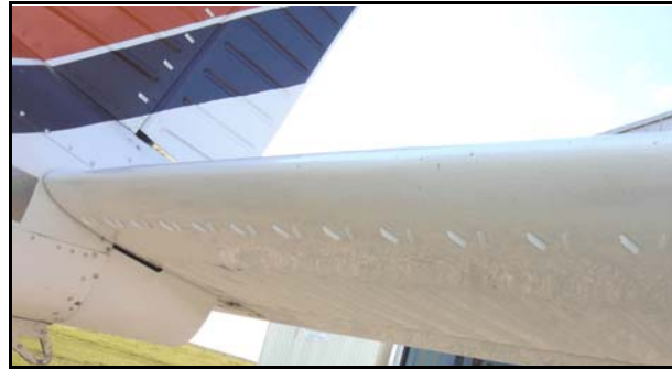
The VGs are installed on the bottom of the stabilator and up the trailing edge of the vertical stabilizer.
